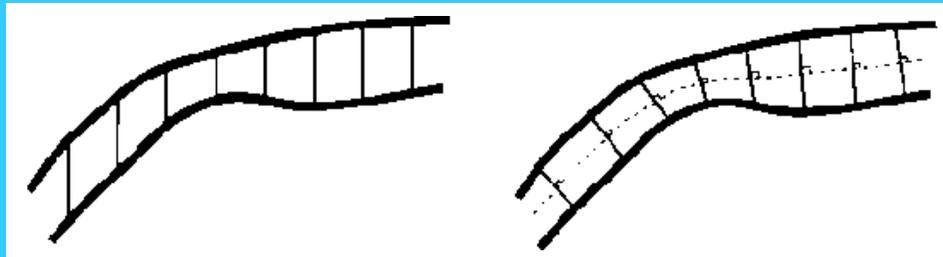
Two approaches to establish areal gridding: (1) on the left, the cells/nodes are stacked vertically, and (2) on the right, the cells/nodes are aligned on lines perpendicular to the bounding surfaces. The first approach, with a universal vertical coordinate, is preferred because of computational simplicity.
